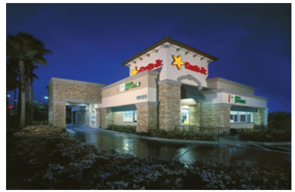
After an electrical fire destroyed the face of a Carl's Jr. fast-food franchise sign, the neon signage was replaced with new LED signage powered by LED drivers. Input watts dropped from 200W to 38W with the LED system, producing a payback in less than two years. (Photo courtesy of Advance Transformer Co.)
